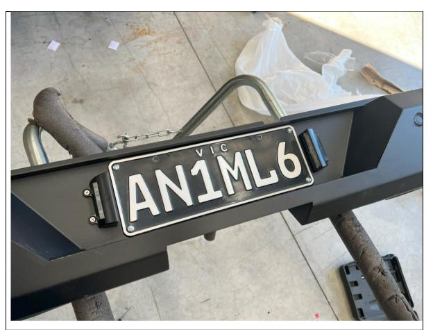
55. Re-Fit number plate to the bar, using supplied M5 Fasteners.
