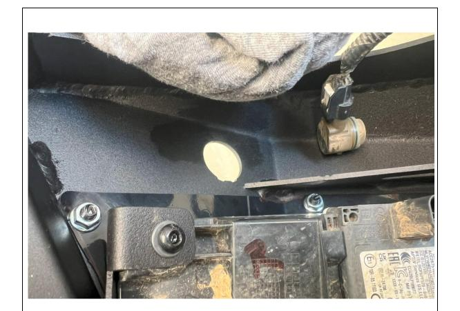
35. Clean areas adjacent to parking sensor locations on inside of bar with isopropyl alcohol.
