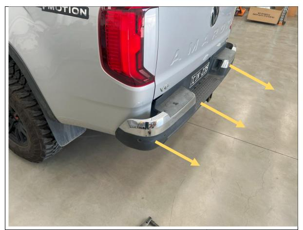
6. With all fasteners removed and the factory bumper assembly free, remove the bumper from the vehicle in a rearward direction.
