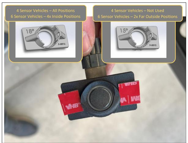
38. Determine correct sensor housings for each sensor location.
