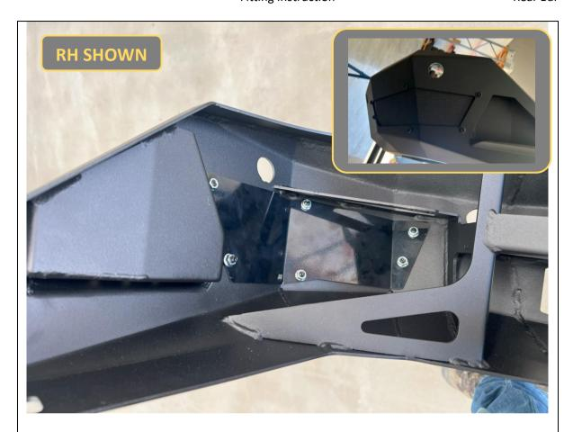
28. Fit the plastic radar covers to the **INSIDE** of the rear radar window, using supplied M6x16 Button Head bolts, Flat washers, and Flange Nuts.
